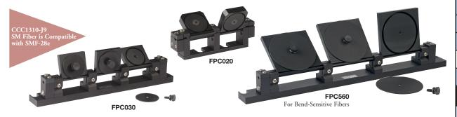
If your application includes single mode fiber and requires linearly polarized light, the FPC Series of Polarization Controllers can be easily implemented to convert elliptically polarized light in a single mode fiber into another state of polarization, including linearly polarized light. This polarization conversion is achieved by loading the paddles with a prescribed number of fiber loops and adjusting their positions to control the output polarization state.
