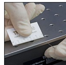
Click to Enlarge Cleaving Fiber Optic Cannula with the CSW12-5
