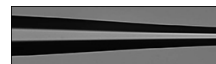
Click to Enlarge Ø20 µm core, Ø400 µm cladding large-mode-area (LMA) fiber tapered to Ø125 µm cladding.
